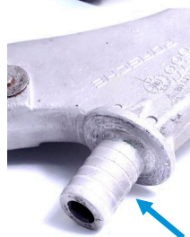
Clean shaft Surface. Figure 1
