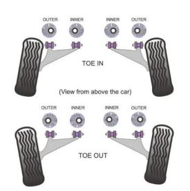
Hole positions in the sleeves, looking at them from the outside of the car on both sides, showing maximum adjustment limits. The adjusters will have to be adjusted individually to achieve the desired toe and camber settings.
