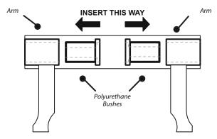
Figure 1 - Positioning of Polyurethane Bushes
