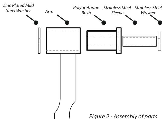
Figure 2 - Assembly of parts
